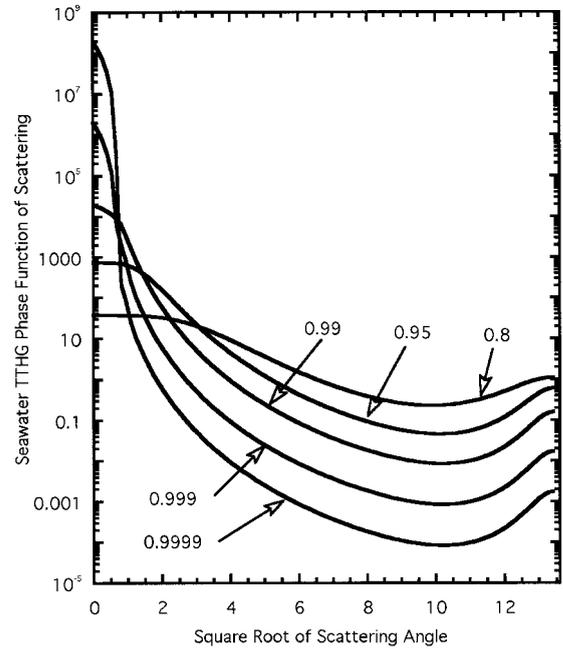
Fig. 2. Samples of marine TTHG phase functions for different values of asymmetry parameter  $g$ .
