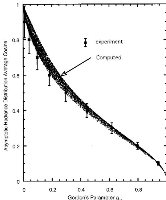
Fig. 4. Comparison of average cosines of the asymptotic radiance distribution computed for all possible combinations of  $B$  and  $\omega_0$  with the experimental average cosines plotted against Gordon's parameter  $g_x = B\omega_0/(1 - \omega_0 + B\omega_0)$ .
