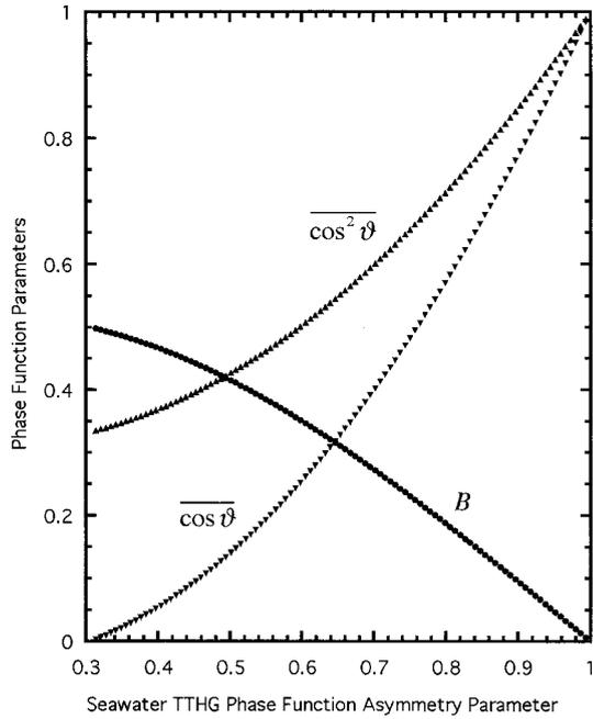
Fig. 1. Dependence of integral parameters ( $B$ ,  $\overline{\cos \vartheta}$ ,  $\overline{\cos^2 \vartheta}$ ) of the marine TTHG phase function on asymmetry parameter  $g$ .
