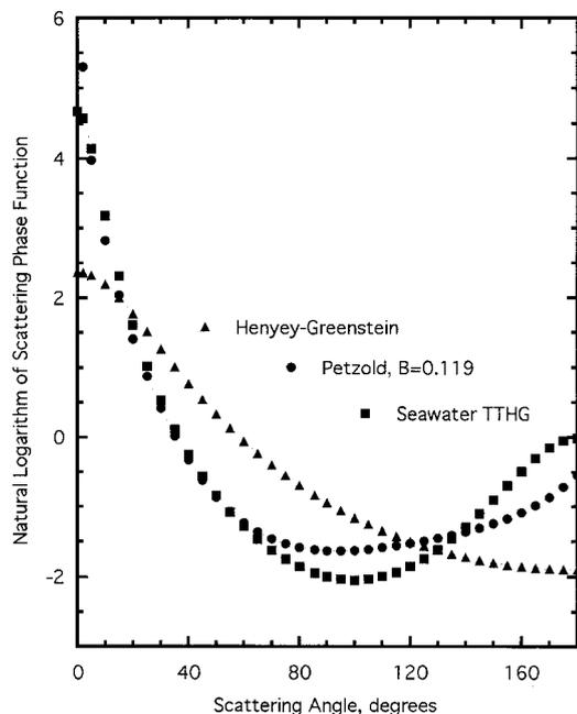
Fig. 3. Comparison of the HG phase function, the one-parameter seawater TTHG phase function, and the experimental Petzold phase function<sup>7</sup> with the same value of backscattering probability  $B = 0.119$ .
